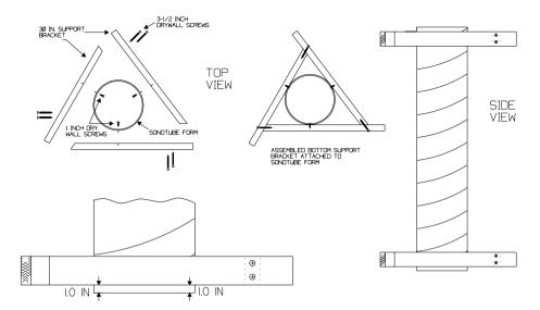
STEP #5 ATTACHMENT OF THE LOWER ADJUSTMENT BRACKETS
