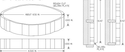
MODIFICATION #1 - CHUCK THE ROUGHCUT DELRIN PLATE IN A LATHE AND TURN AS MUCH OF THE OF THE OUTER EDGE AS POSSIBLE TO A DIAMETER OF ABOUT 6.0 INCHES. FLIP THE PLATE IN THE LATHE CHUCK AND TURN THE REMAINDER OF THE EDGE TO 6.00 INCHES. WHILE THE PLATE IS STILL IN THE LATHE. MARK THE CENTER OF THE PLATE.
