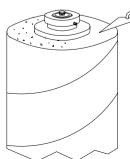
USE A TROWEL TO SMOOTH THE TOP OF THE CONCRETE. IF POSSIBLE. TRY TO SLOPE IT TO THE OUTER EDGE SO THAT WATER WILL RUN OFF. BE CAREFUL NOT TO DISTURB ANTENNA MOUNT.
