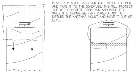
THIS COMPLETES THE INTITIAL SETTING OF THE RECOMMENDED CORS MONUMENT. THE FOLLOWING STEPS ARE TO BE DONE AFTER THE CONCRETE HAS CURED FROM 3 TO 7 DAYS.
