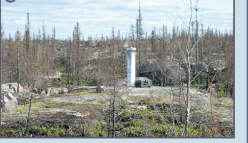
FIGURE 1. Location of select regional sites of the Canadian Base Network, initiated in 1994. The CBN is a national network of pillar monuments with forced-centering plates for Global Positioning System (GPS) receiver antennae. The GPS sites with co-located absolute gravity (AG) observations are indicated.
