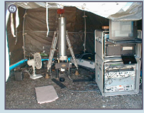
FIGURE 5. JILA-2 absolute gravimeter at La Grande-1 (James Bay Region, Quebec). Acquired in late 1985, the JILA-2 operates by using the free-fall method. This instrument has been upgraded three times since its acquisition with new computer control, new lasers, GPS clock and ancillary equipment. These upgrades were necessary in order to make it more efficient, field-worthy, lighter and easier to use. For the sites of the James Bay/Novelle Quebec Region, JILA-2 is generally operated within a tent in an often challenging environment.
