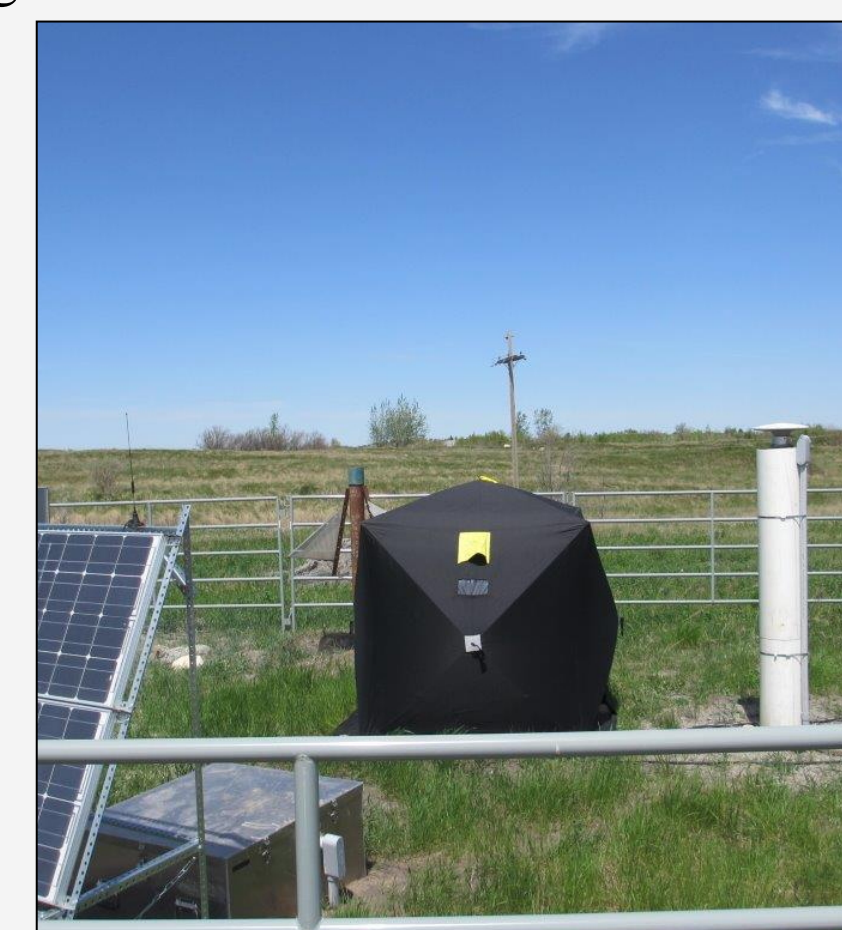
Fig 6: InSAR Pillar w/ GPS
